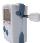
Once your KISTOCK is set on the mounting plate, insert the key to lock the mounting system.
